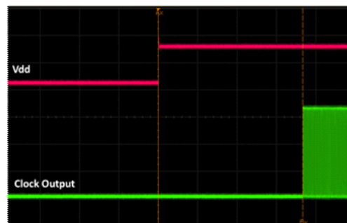
Figure 17. Startup Waveform vs. Vdd
