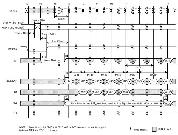
Figure 0 - VDD/VDDQ Voltage Switch Between DDR3L and DDR3L
