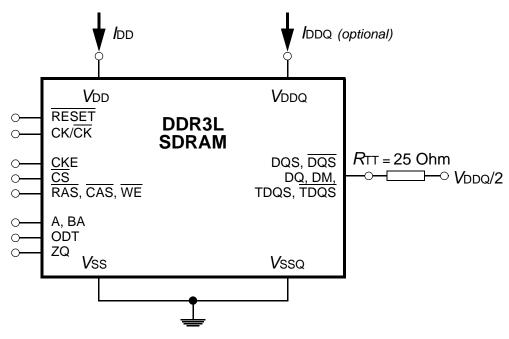
Figure 1 - Measurement Setup and Test Load for IDD and IDDQ (optional) Measurements [Note: DIMM level Output test load condition may be different from above]
