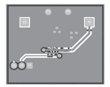
Figure 4: AAT2113B Evaluation Board Bottom Side Layout for 1.2V Fixed Output Voltage Version.
