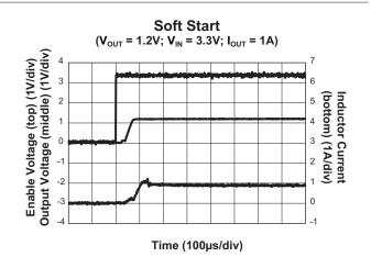
Soft Start  $(V_{OUT} = 2.5V; V_{IN} = 3.3V; I_{OUT} = 1A)$ Output Voltage (middle) (1V/div) 4 7 Enable Voltage (top) (1V/div) 3 6 (bottom) (1A/div) 2 Inductor Current 5 4 1 3 0 2 -1 -2 1 -3 0 -4 Time (100µs/div)
