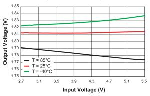
Output Voltage vs. Input Voltage (V<sub>OUT</sub> = 2.5V; I<sub>OUT</sub> = 1A)
