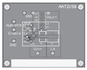
Figure 3: AAT2158 Evaluation Board Top Side Layout.
