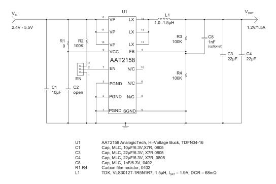
Figure 2: AAT2158 Alternate Application Schematic.
