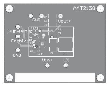
Figure 4: AAT2158 Evaluation Board Bottom Side Layout.
