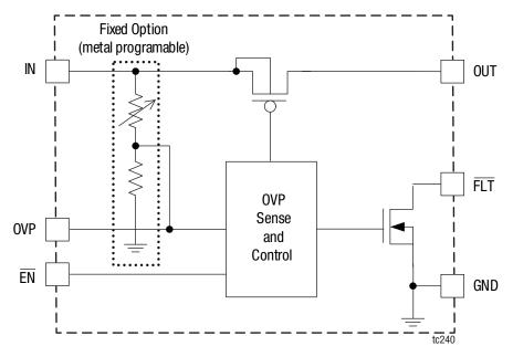
Figure 21. AAT4687 Functional Block Diagram
