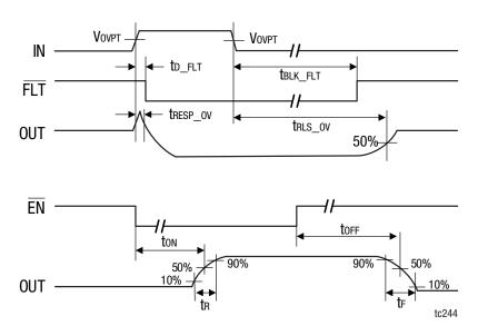
Figure 22. AAT4687 Timing Diagram
