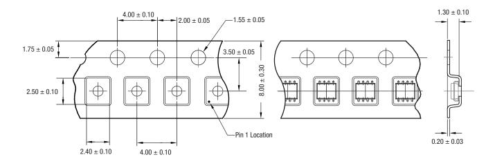
Figure 29. AAT4687 10-pin SC70JW Tape and Reel Dimensions
