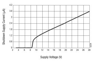
Figure 5. Shutdown Supply Current vs Supply Voltage
