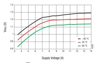
Figure 16. EN Input Low Voltage vs Supply Voltage
