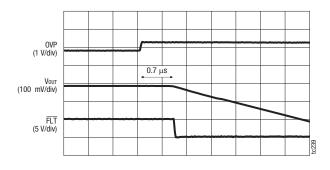
Figure 25. Typical Over-Voltage Response (Zoom View)
