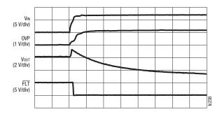
**Figure 19. Over-Voltage Protection Response**
