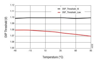
Figure 13. Over-Voltage Lockout Threshold vs Temperature
