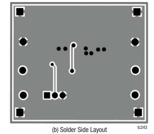
Figure 27. AAT4687 Evaluation Board Layer Details
