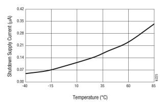
Figure 6. Shutdown Supply Current vs Temperature (VIN = 6.5 V)
