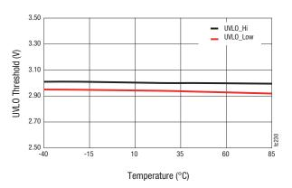
Figure 11. Under-Voltage Lockout Threshold vs Temperature
