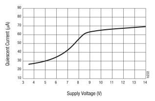
**Figure 3. Operation Quiescent Current vs Supply Voltage**
