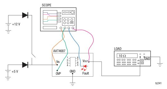
Figure 23. Over-Voltage Protection Response Time Test Circuit
