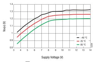
Figure 15. EN Input High Voltage vs Supply Voltage
