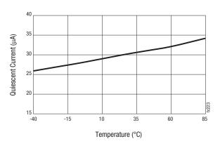
Figure 4. Operation Quiescent Current vs Temperature (VIN = 5 V, No Load)
