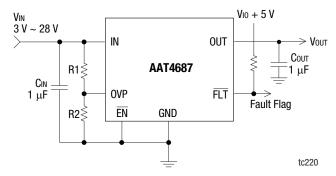
Figure 1. AAT4687 Typical Application Circuit
