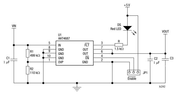
Figure 26. AAT4687 Evaluation Board Schematic
