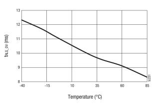
Figure 12. Over-Voltage Release Time vs Temperature (VIN = 5 V, Cout = 1  $\mu$ F, Rout = 10  $\Omega$ )
