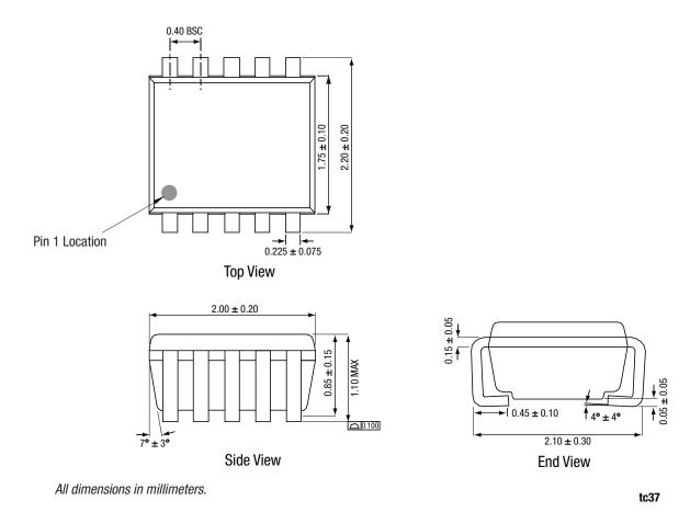
Figure 28 AAT4687 10-pin SC70JW Package Dimensions
