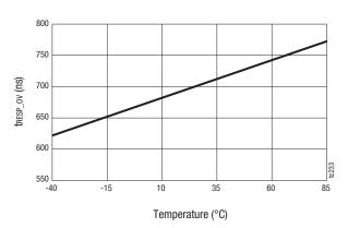
Figure 14. Over-Voltage Response Time vs Temperature
