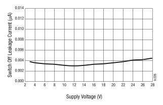
Figure 7. Switch Off Leakage vs Supply Voltage
