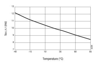
Figure 10. FLT Blanking Time vs Temperature
