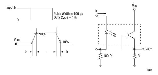
Figure 5. OLI249 Switching Test Circuit
