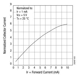
**Figure 3. Normalized Collector Current vs Forward Current**
