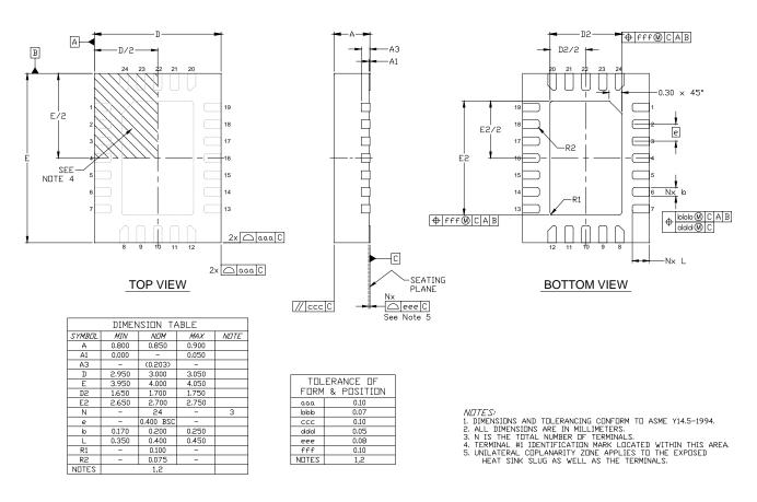
Figure 5. SE2431L Package Dimensions
