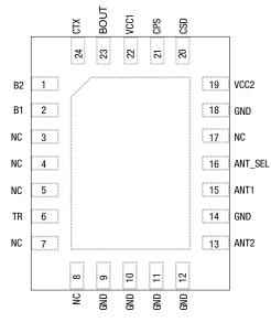
Figure 2. SE2431L Pinout (Top View)
