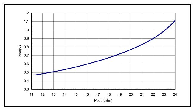
Figure 3: SE2614BT Power Detector Characteristics
