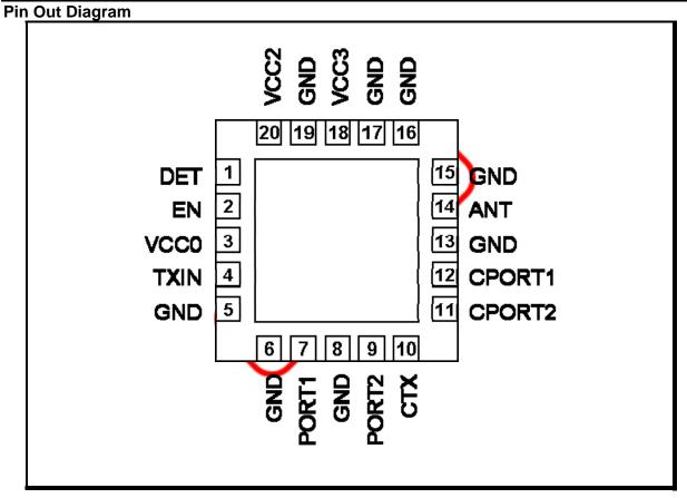
Figure 2: SE2614BT Pin Out (Top View Through Package)
