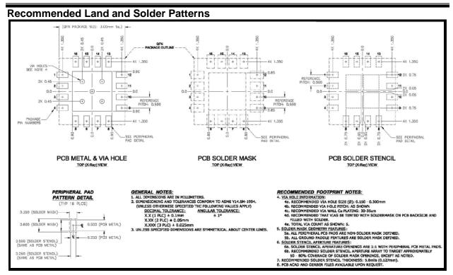
Figure 5: SE5007BT Recommended Land and Solder Pattern
