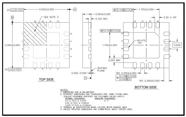
Figure 4: SE5007BT Package Diagram
