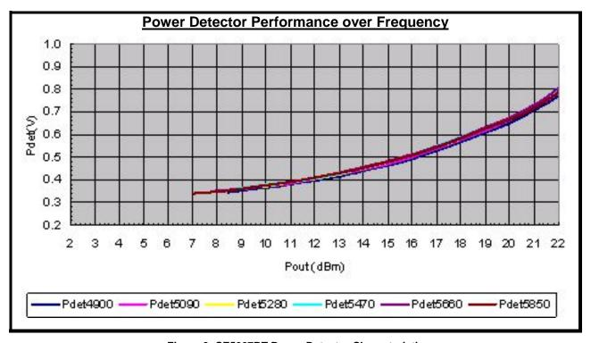
Figure 3: SE5007BT Power Detector Characteristic
