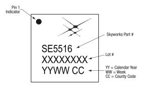
Figure 8. Typical Part Markings (Top View)
