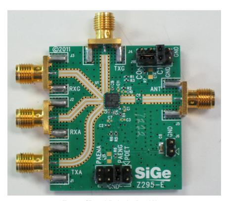
Figure 6. SE5516A Evaluation Board Photo
