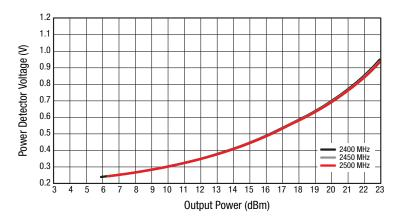
Figure 3. Power Detector vs Output Power Over Frequency
