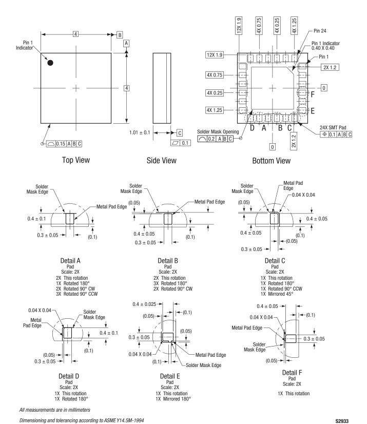
Figure 9. SE5516A Package Dimensions
