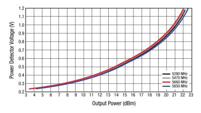
Figure 4. Power Detector vs Output Power Over Frequency @ 5.0 GHz
