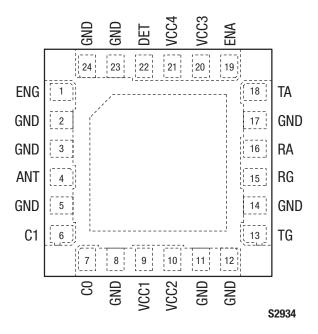
Figure 2. SE5516A Pinout (Top View)
