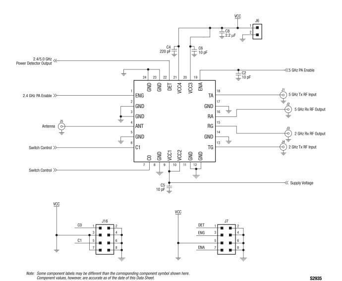
**Figure 5. SE5516A Evaluation Board Schematic**
