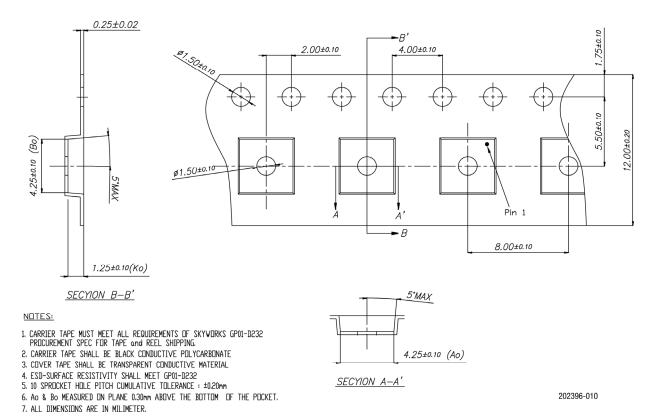
Figure 10. SE5516A Tape and Reel Dimensions
