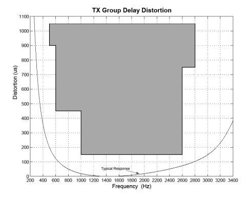
Figure 3.9. Transmit Group Delay Distortion
