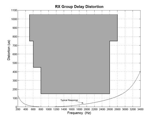
Figure 3.10. Receive Group Delay Distortion
