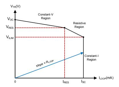
Figure 4.1. Dual ProSLIC DC Feed Characteristics
