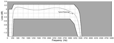
Figure 3.8. Transmit Path Frequency Response
