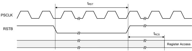
Figure 3.1. Reset Timing Diagram
