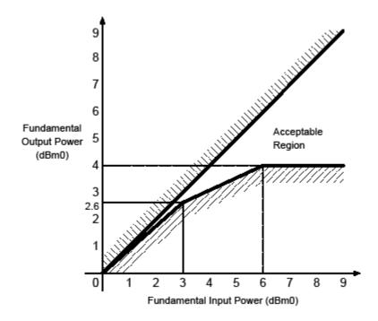
Figure 3.6. Overload Compression Performance
