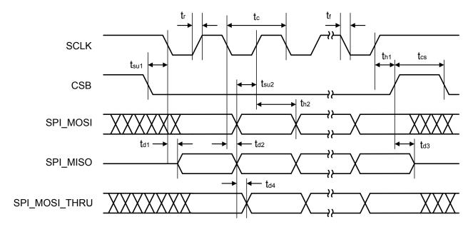
Figure 3.2. SPI Timing Diagram
