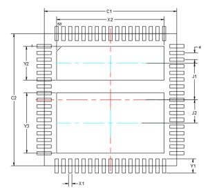
Figure 7.2. 68-Pin QFN Land Pattern
