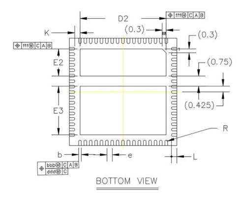
Figure 7.1. 68-Pin QFN Package
