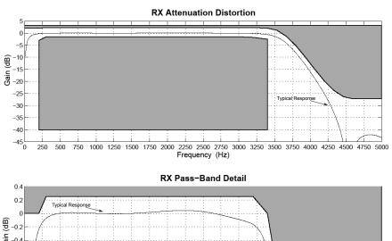
Figure 3.7. Receive Path Frequency Response
