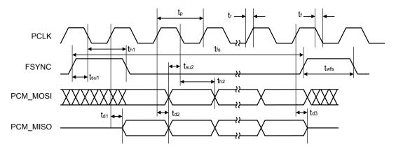
Figure 3.3. PCM Highway Interface Timing Diagram
