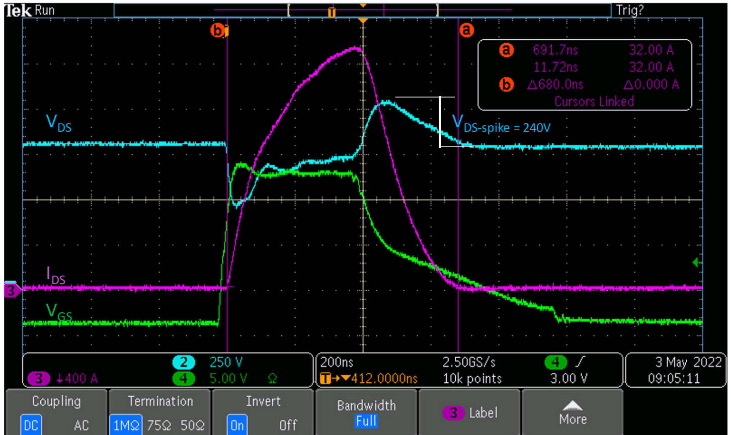
Figure 5.4. Si8285 DESAT Waveform with V_{Rail} = 800 V, R_{SS} = 22 \Omega , and C3M0016120K SiC
