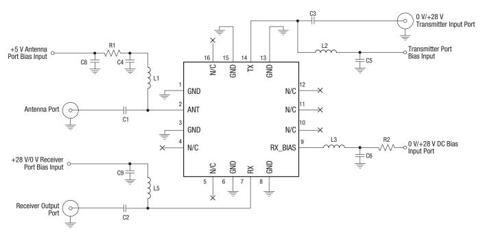
NOTE: The N/C pins (4, 5, 10, 11, 12, and 16) are not internally connected, so they can be left open or grounded.
