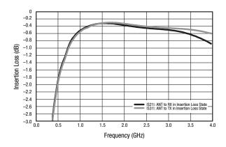
Figure 4. Insertion Loss vs Frequency (ANT to RX and ANT to TX Ports; VctL = 5 V, IctL = -50 mA)
