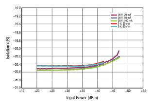
Figure 11. Isolation vs CW Input Power (ANT to RX Port, f = 2.6 GHz)
