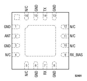
Figure 2. SKY12207-306LF Pinout (Top View)
