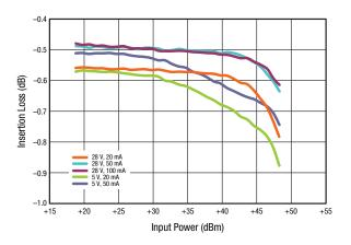
Figure 10. Insertion Loss vs CW Input Power (TX to ANT Port, f = 2.6 GHz)
