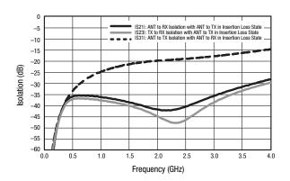
Figure 5. Isolation vs Frequency (ANT to RX, TX to RX, and ANT to TX Ports;  $V_{CTL}=28~V,~I_{CTL}=-50~mA$ )
