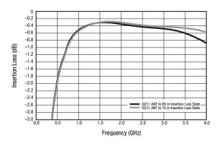
Figure 3. Insertion Loss vs Frequency (ANT to RX and ANT to TX Ports; VctL = 28 V, IctL = -50 mA)
