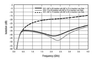
Figure 6. Isolation vs Frequency (ANT to RX, TX to RX, and ANT to TX Ports;  $V_{CTL} = 5 V$ ,  $I_{CTL} = -50 mA$ )
