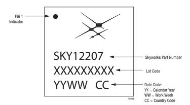
Figure 24. Typical Part Markings
