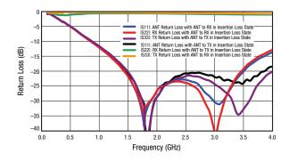
Figure 7. Return Loss vs Frequency (ANT, TX, and RX Ports; Vctl = 28 V, Ictl = -50 mA)
