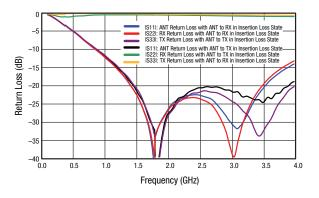
Figure 8. Return Loss vs Frequency (ANT, TX, and RX Ports; Vctl. = 5 V, Ictl. = -50 mA)
