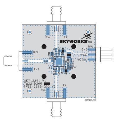
Figure 10. SKY12241-492LF Evaluation Board Assembly Diagram
