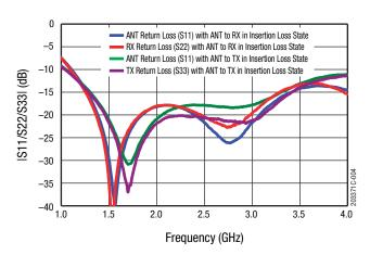
**Figure 4. Return Loss vs Frequency**
