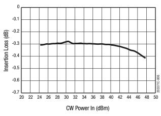
Figure 6. Insertion Loss vs CW Input Power (ANT-TX, f = 2.6 GHz)
