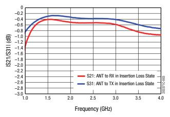
**Figure 3. Insertion Loss vs Frequency**
