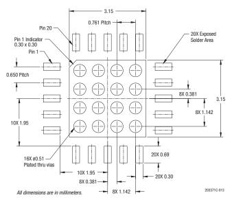
**Figure 13. PCB Layout Footprint**
