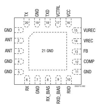
Figure 2. SKY12241-492LF Pinout (Top View)
