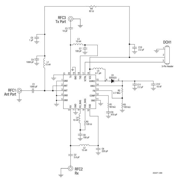
Figure 9. SKY12241-492LF Evaluation Board Schematic
