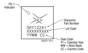
Figure 14. Typical Part Markings (Top View)
