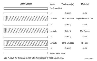
Figure 12. SKY12241-492LF Layer Detail Physical Characteristics
