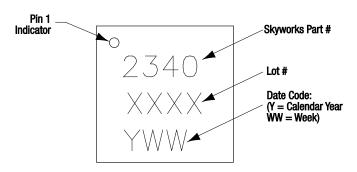
Figure 18. Typical Part Markings
