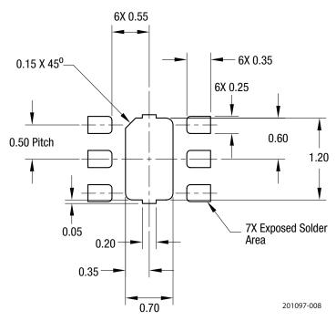
Figure 8. SKY13320-374LF PCB Layout Footprint (Top View)
