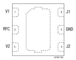
Figure 2. SKY13320-374LF Pinout (Top View)
