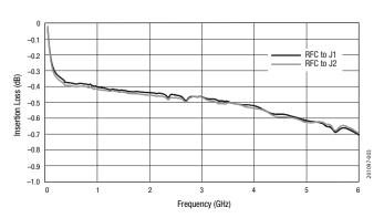
**Figure 3. Typical Insertion Loss**
