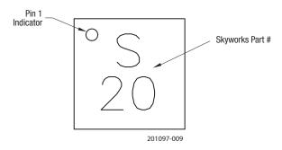
Figure 9. Typical Part Markings (Top View)
