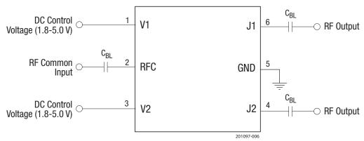
C<sub>BL</sub> = 47 pF for >1 GHz operation. Exposed ground paddle should be grounded for best performance.
