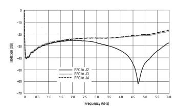
Figure 4. Isolation vs Frequency (RFC to J1 Insertion Loss State)
