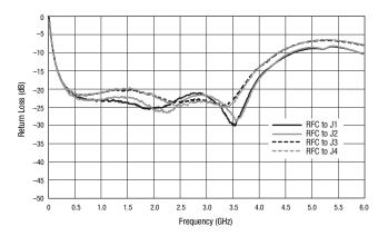
Figure 8. RFC Return Loss vs Frequency
