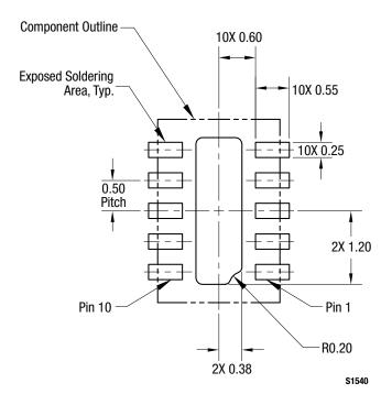
Figure 11. SKY13322-375LF PCB Layout Footprint (Top View)
