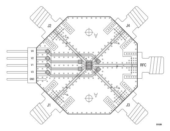
Figure 10. SKY13322-375LF Evaluation Board Assembly Diagram
