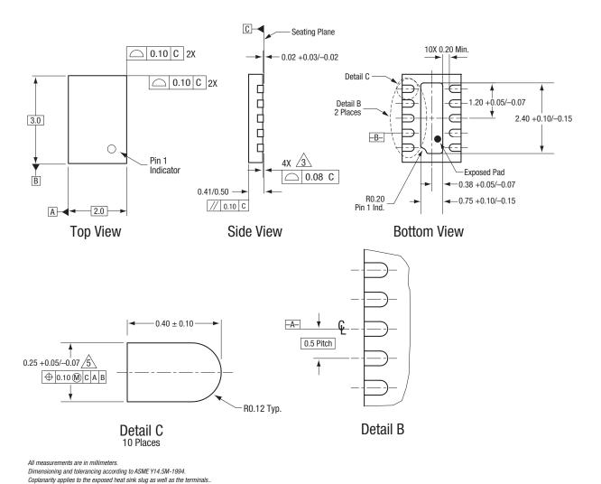
Figure 13. SKY13322-375LF 6-Pin QFN Package Dimensions
