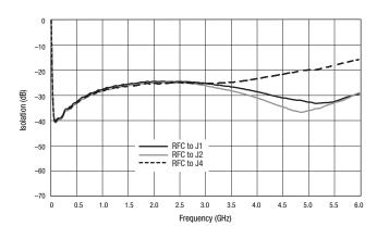
Figure 6. Isolation vs Frequency (RFC to J3 Insertion Loss State)
