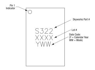
Figure 12. Typical Case Markings (Top View)
