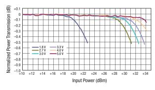
Figure 6. Compression vs Control Voltage (2450 MHz)
