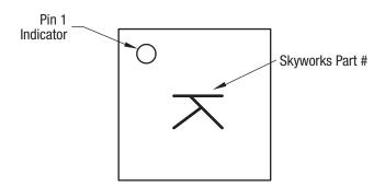
Figure 13. Typical Part Markings (Top View)
