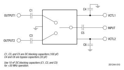
Figure 10. SKY13366-378LF Evaluation Board Schematic
