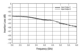
**Figure 3. Typical Insertion Loss**
