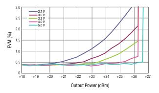
Figure 8. 802.11g EVM vs Output Power @ 2.45 GHz, 54 Mbps
