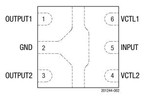
Figure 2. SKY13366-378LF Pinout (Top View)
