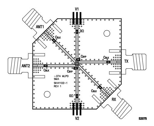
Figure 8. SKY13381-374LF Evaluation Board Assembly Diagram
