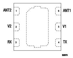
Figure 2. SKY13381-374LF Pinout – 6-Pin MLPD (Top View)
