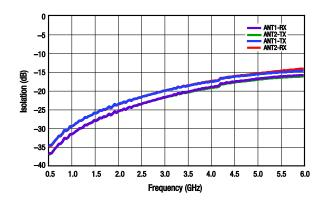
Figure 4. Isolation vs Frequency (ANT1/ANT2 to TX/RX)
