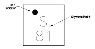
Figure 10. Typical Part Markings (Top View)
