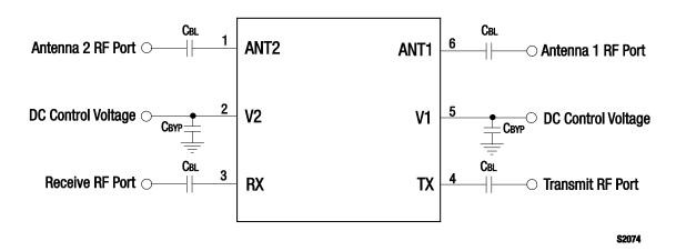
Figure 7. SKY13381-374LF Evaluation Board Schematic
