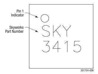
Figure 6. Typical Part Markings (Top View)
