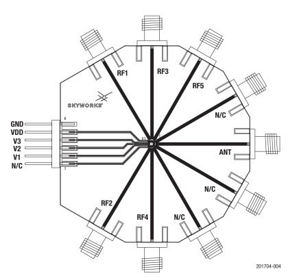
Figure 4. SKY13415-485LF Evaluation Board Assembly Diagram
