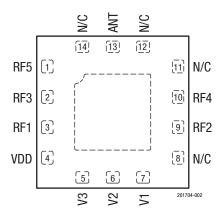
Figure 2. SKY13415-485LF Pinout (Top View)
