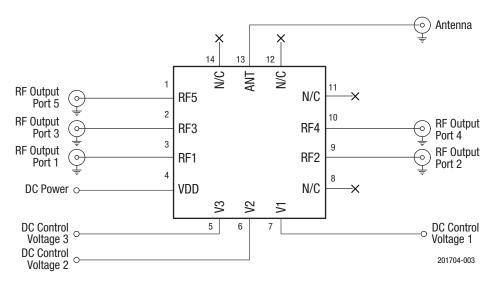
Figure 3. SKY13415-485LF Evaluation Board Schematic
