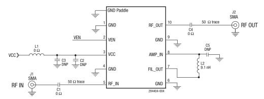
Figure 4. SKY65943-11 Evaluation Board Schematic
