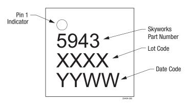
Figure 6. Typical Part Markings (Top View)
