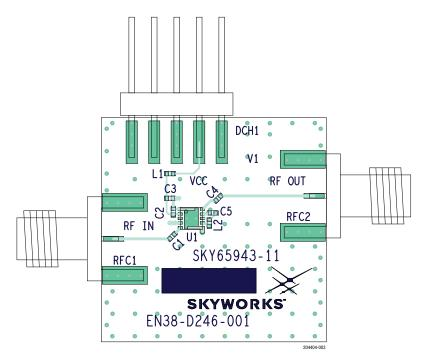
Figure 3. SKY65943-11 Evaluation Board Assembly Diagram
