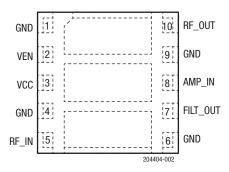
Figure 2. SKY65943-11 Pinout (Top View)
