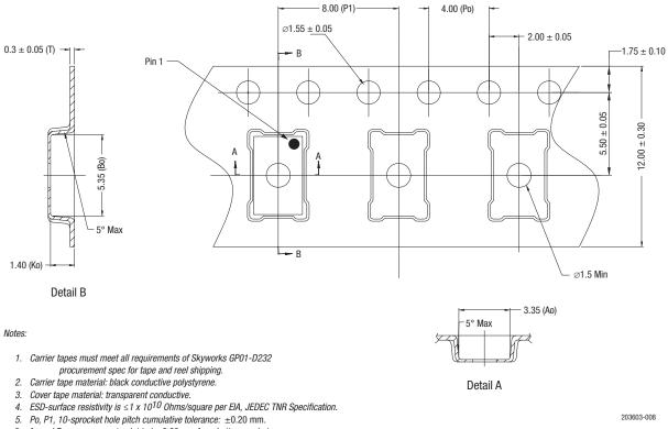
6. Ao and Bo measurement point to be 0.30 mm from bottom pocket.
