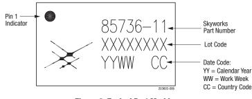
Figure 6. Typical Part Markings (Top View)
