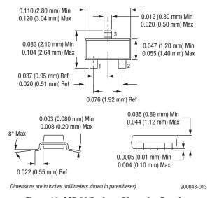
Figure 11. SOT-23 Package Dimension Drawing
