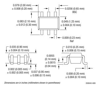
Figure 7. SC-88 Package Dimension Drawing
