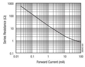
Figure 1. Series Resistance vs Current @ 100 MHz
