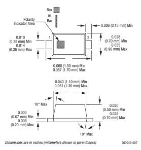
Figure 5. SC-79 Package Dimension Drawing
