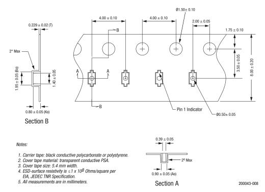
Figure 6. SC-79 Tape and Reel Dimensions
