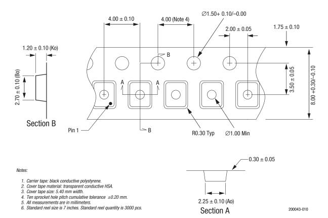
Figure 8. SC-88 Tape and Reel Dimensions
