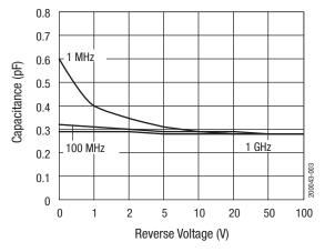
Figure 3. Capacitance vs Reverse Voltage
