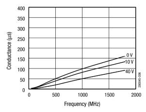
Figure 6. Conductance vs Frequency and Reverse Voltage
