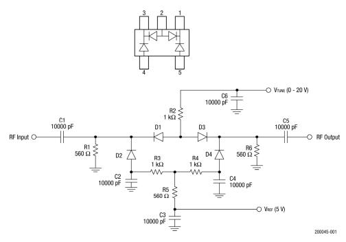
Figure 1. SMP1307-027LF Application Circuit
