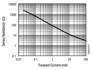
Figure 3. Series Resistance vs Current @ 100 MHz
