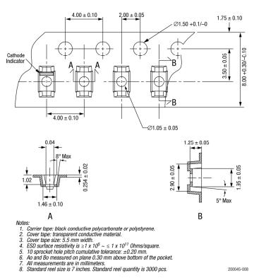
Figure 8. SOD-323 Tape and Reel Dimensions
