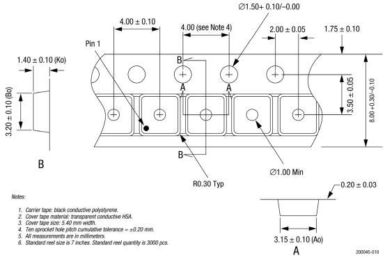
Figure 10. SOT-5 Tape and Reel Dimensions
