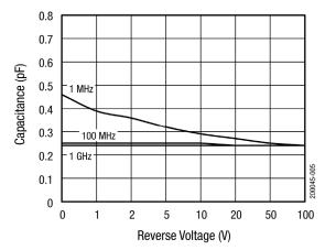
Figure 5. Capacitance vs Reverse Voltage
