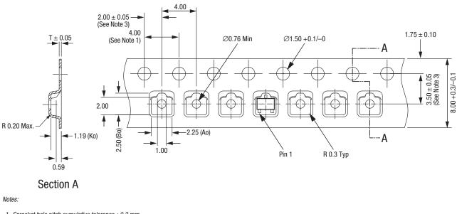
1. Sprocket hole pitch cumulative tolerance  $\pm 0.2$  mm.
