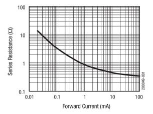
Figure 1. Series Resistance vs Current @ 100 MHz
