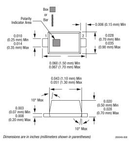
Figure 7. SC-79 Package Dimension Drawing
