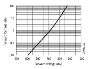
**Figure 2. Forward Current vs Voltage**
