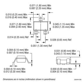
Figure 5. SC-70 Package Dimension Drawing
