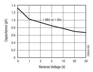
Figure 3. Capacitance vs Reverse Voltage
