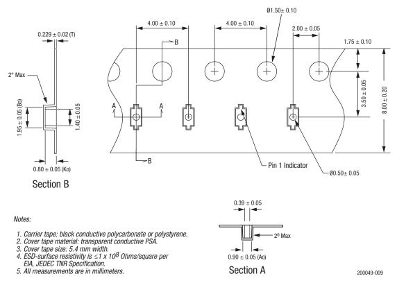
Figure 8. SC-79 Tape and Reel Dimensions
