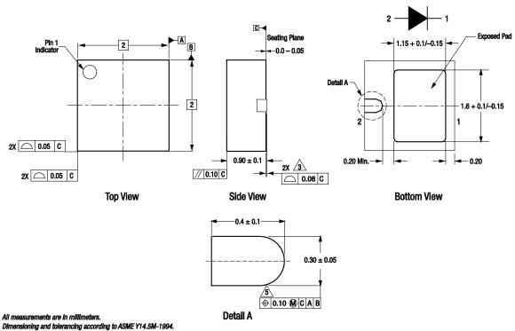
Dimensioning and tolerancing according to ASME Y14.5M-1994.
