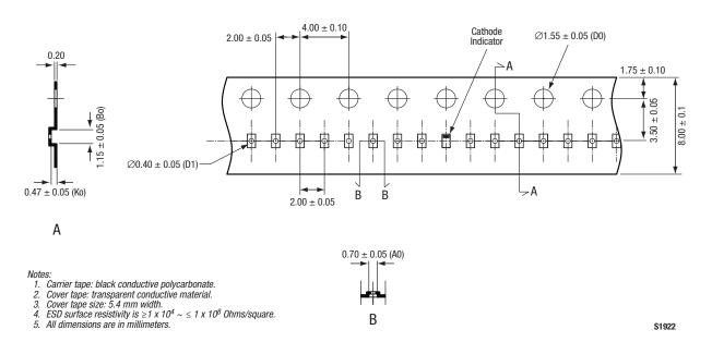
Figure 10. SOD-882 Tape and Reel Dimensions
