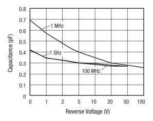
Figure 3. Capacitance vs Reverse Voltage
