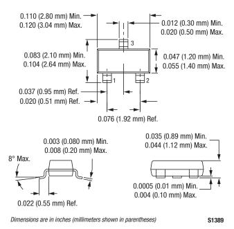
Figure 7. SOT-23 Package Dimension Drawing
