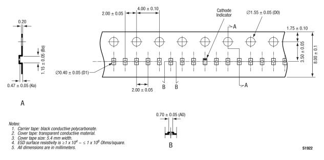
Figure 4. SOD-882 Tape and Reel Dimensions
