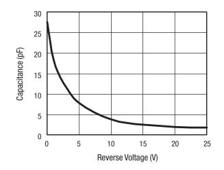
Figure 1. Capacitance vs Reverse Voltage
