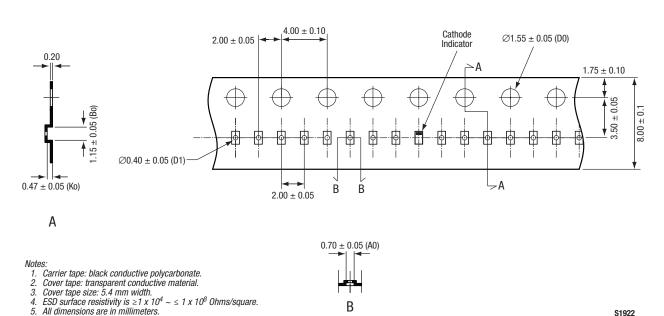
Figure 6. SOD-882 Tape and Reel Dimensions
