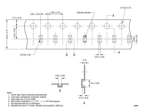
Figure 4. SC-79 Tape and Reel Dimensions
