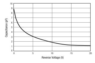
Figure 1. Capacitance vs Reverse Voltage
