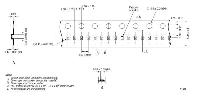
Figure 7. SMV2025-040LF Tape and Reel Dimensions (SC-79)
