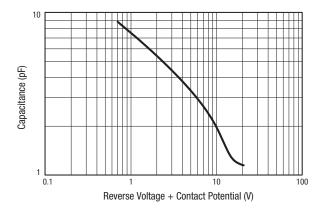
Figure 2. Capacitance vs Reverse Voltage (Logarithmic Plot)
