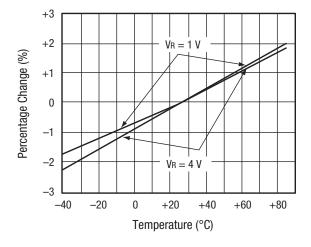
Figure 1. Relative Capacitance Change vs Temperature
