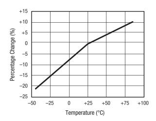
Figure 2. Relative Series Resistance Change vs Temperature @ 500 MHz
