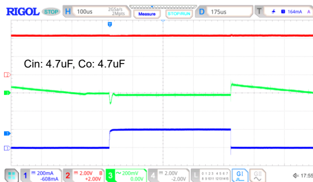
V_{IN}=4.3V, V_{OUT}=3.3V I_{OUT}=1mA to 200mA
