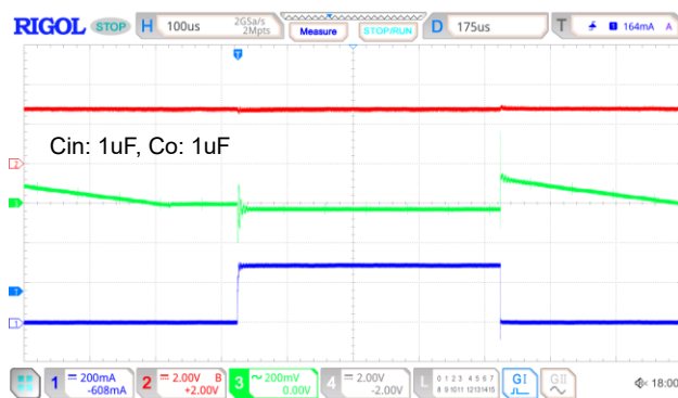
V_{IN}=2.8V, V_{OUT}=1.2V I_{OUT}=1mA to 300mA
