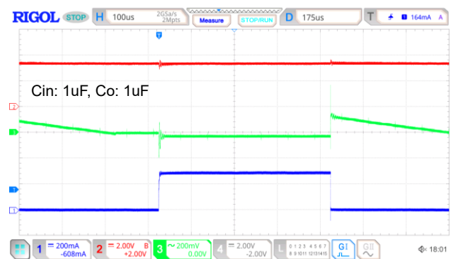
V_{IN}=3.3V, V_{OUT}=1.2V I_{OUT}=1mA to 300mA
