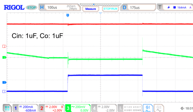
V_{IN}=4V, V_{OUT}=1.2V I_{OUT}=1mA to 300mA
