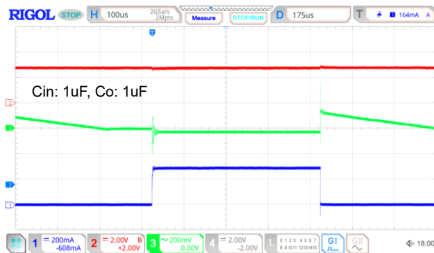
V_{IN}=2.8V, V_{OUT}=1.2V I_{OUT}=1mA to 300mA
