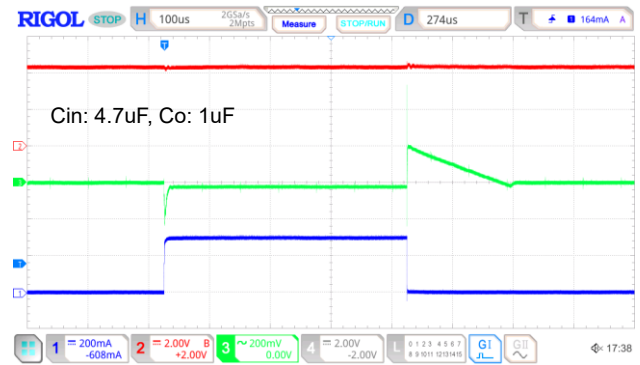
V_{IN}=4.3V, V_{OUT}=3.3V I_{OUT}=1mA to 300mA
