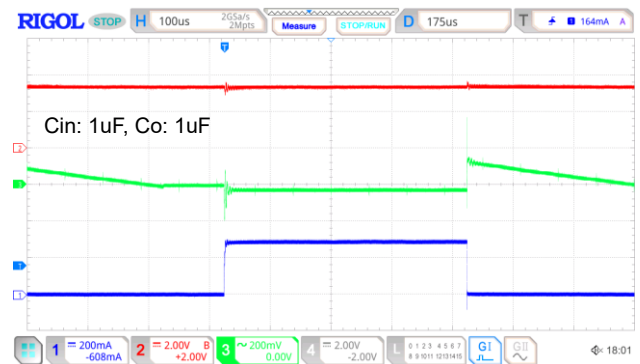
V_{IN}=3.3V, V_{OUT}=1.2V I_{OUT}=1mA to 300mA
