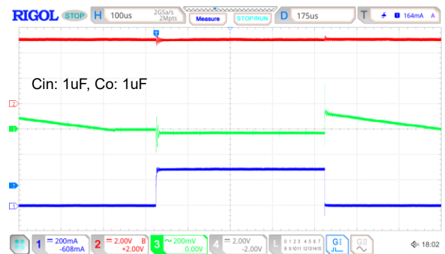
V_{IN}=5V, V_{OUT}=1.2V I_{OUT}=1mA to 300mA
