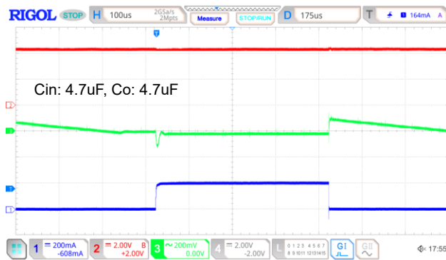
V_{IN}=4.3V, V_{OUT}=3.3V I_{OUT}=1mA to 200mA
