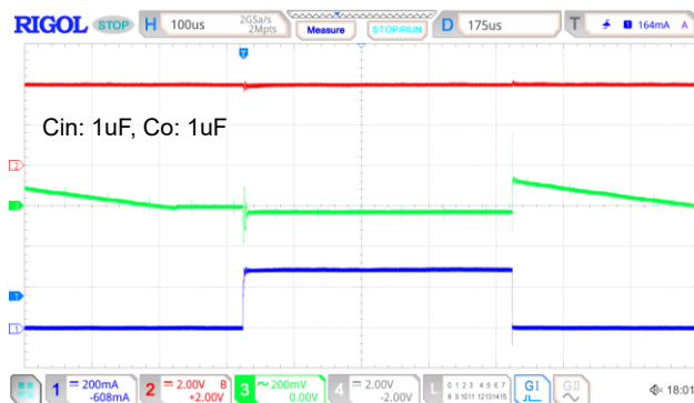
V_{IN}=4V, V_{OUT}=1.2V I_{OUT}=1mA to 300mA
