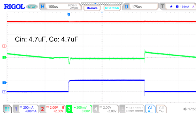
V_{IN}=4.3V, V_{OUT}=3.3V I_{OUT}=1mA to 200mA
