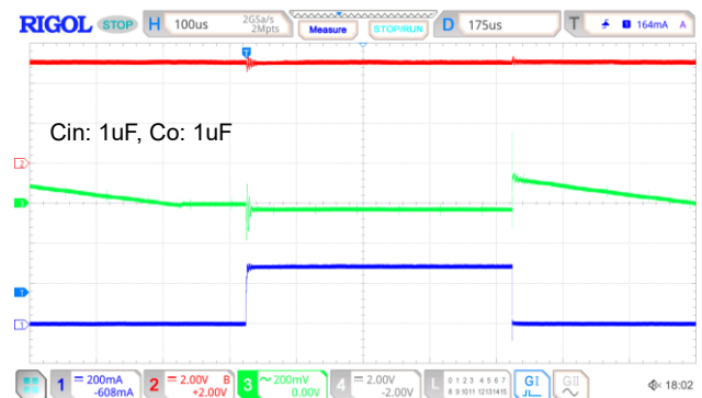
V_{IN}=5V, V_{OUT}=1.2V I_{OUT}=1mA to 300mA
