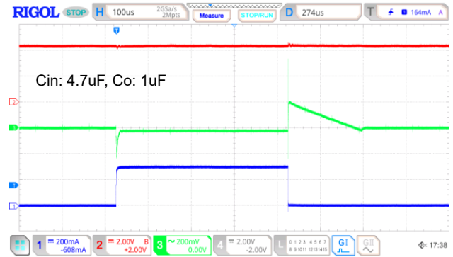
V_{IN}=4.3V, V_{OUT}=3.3V I_{OUT}=1mA to 300mA
