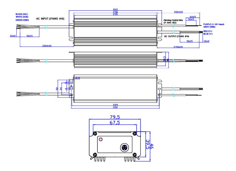
**Dimming Control** The dimming function shown below uses an internal pull-up resistor, with the output at full load when the dimming leads are not connected (floated).
