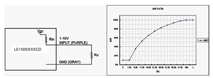
**Dimming Configuration using External Resistance**
