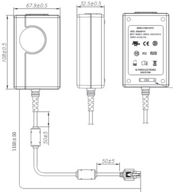
See Note 3: 9V through 48V Models: 2.5 x 5.5 x 9.5mmor equiv. Barrel Connector, center positive<sup>2</sup>
