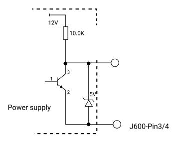
PF/DC OK: During normal operation stays HIGH -goes HIGH 100mS-500mS after main output -goes LOW with 5mS warning before loss of output from AC failure
