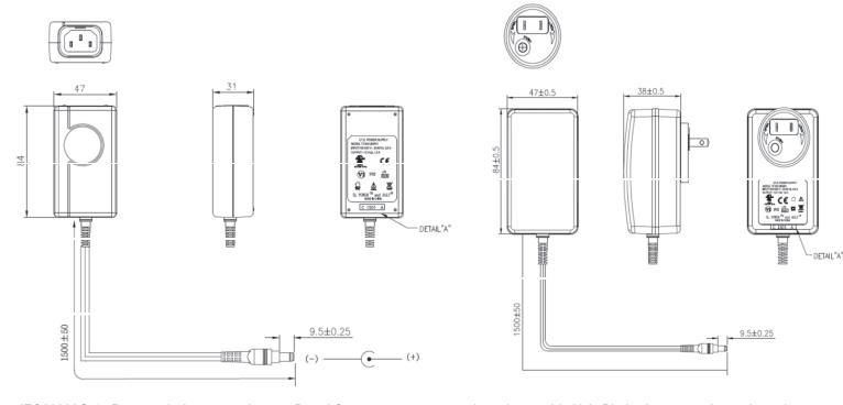
IEC60320C 14 Receptacle, 2 .5 x5 .5 x9 .5mm Barrel Connector
