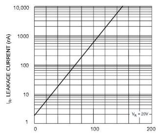
T<sub>i</sub>, JUNCTION TEMPERATURE (°C) Fig. 2, Leakage Current vs Junction Temperature
