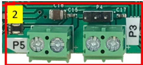
Figure 3 - 12 V power supply connection
