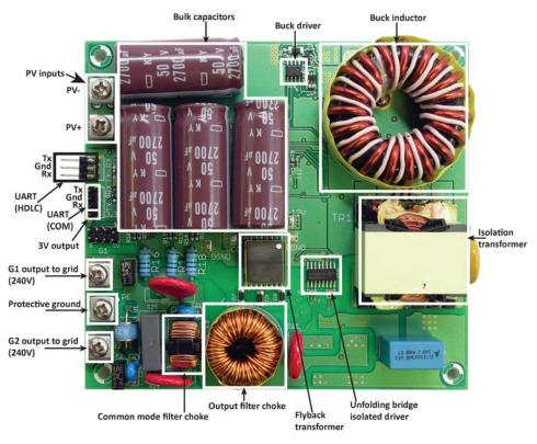
Figure 3 - MI-P300A Development Platform bottom view
