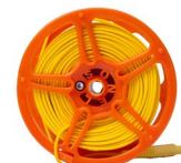
Test lead for earth resistance measurement 50 m
