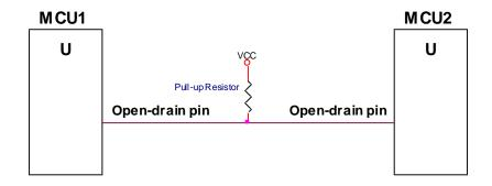
The pull-up resistor is necessary. Open-drain output high is driven by pull-up resistor. Output low is sunken by MCU's pin.
