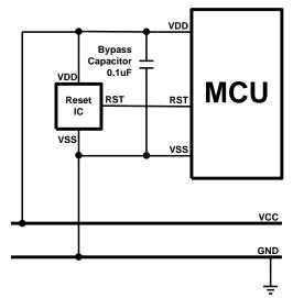
The external reset circuit also use external reset IC to enhance MCU reset performance. This is a high cost and good effect solution. By different application and system requirement to select suitable reset IC. The reset circuit can improve all power variation.
