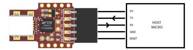
The microUSB is designed to have a compact footprint, and be compatible with prototyping such as plugging it directly into a breadboard when male 2.54mm (0.1") headers are soldered to the row of 5 pins, along each side.
