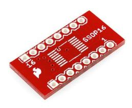
**Description:** 8, 16, 20, and 28-Pin SSOP to DIP break out boards. The footprint was rotated to accommodate different width SSOP devices and can be used with any pin count up to 28 pins. Designed to be used with 0.65mm pitch devices but can also be used with 0.025" pitch devices (comes out to  $\sim$ 0.635mm). We've made these 0.635mm devices fit just fine. Can be used with packages from 0.200" (5mm) up to 0.450" (11.4mm) in width.
