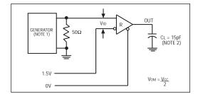
Figure 6. Receiver Propagation Delay Test Circuit
