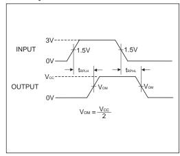
Figure 11. Receiver Propagation Delay Waveforms
