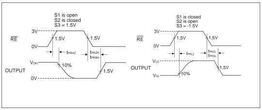
Figure 12. Receiver Enable and Disable Waveforms
