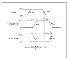
Figure 8. Driver Propagation Delay Waveforms
