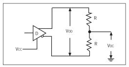
Figure 1. Driver DC Test Load Circuit
