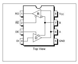
SP3481/SP3485 Pinout (Top View)
