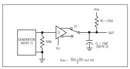
Figure 2. Driver Propagation Delay Test Circuit
